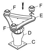
Place the Pedestal (D) upside side. Tighten the Mounting plate (C) to Table top(A) by bolt(G), lock washers (H) and flat washers (I) with allen key (J). Open the lock under Table top(A).
