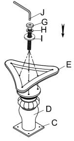
Place the Pedestal (D) upside down . Tighten the Bun Foot (F).
