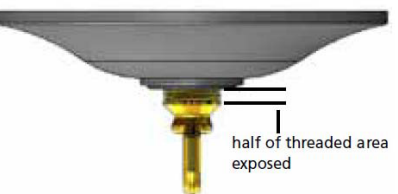
Drawing 2 – Canopy Adjustment
