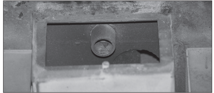
Figure 34: Remove ash from igniter tube (underneath firepot)
