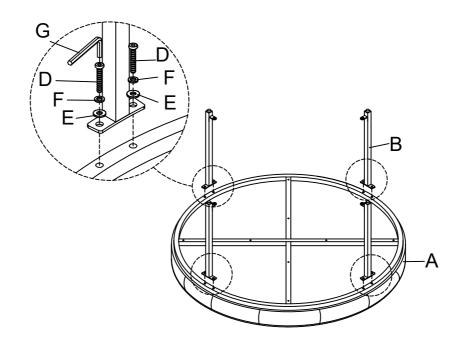
2 Attach Leg (B) to X-Base (C), using Bolt (D), Flat Washer (E) & Lock Washer (F) by Allen Key (G) as below shown.
