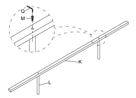
6 Attach Slat (K) to Side Panel (E), (G), (F), (H) using Bolt (N), Lock Washer (O), Flat Washer (P) by Allen Key (Q).
