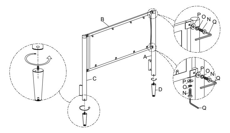
2 Attach Right Side Panel - Front (G) to Right Side Panel - Rear (H) using Bolt (N), Lock Washer (O), Flat Washer (P) by Allen Key (Q).
