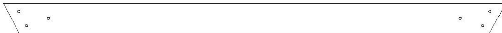
G50 | PLANCHE DE SOL - W4L12330 (x1) | 1 po x 5 1/4 po x 86 3/4 po (24x134x2202)
