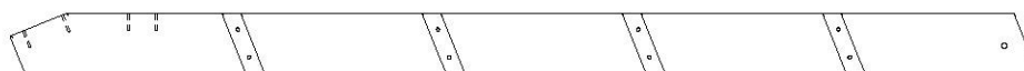
E80 | MONTANT GAUCHE - W4L11751 (x1) | 1-3/8 po x 3-3/8 po x 58 po (36 x 86 x 1474)
