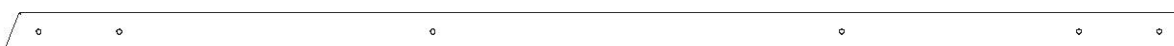
F4 | PLANCHE DE SOL - W4L12487 (x1) | 1-3/8 po x 2-3/8 po x 74-1/8 po (36 x 60 x 1883)
