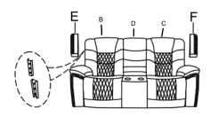
STEP 2:Install the LSF backrest (B), Console back (D), and RSF backrest (C) by align and insert the metal bracket to the metal brackets of the seat (A).Connect the wire between the backrest (B) and backrest (C) with the wires on seat (A).Please make sure the brackets are inserted all the way and secured into position.
