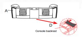
STEP3:Install the LSF backrest (B), Console back (D), and RSF backrest (C) by align and insert the metal br acket to the metal brackets of the seat (A).Please make sure the brackets and console back are inserted all the way and secured into position.
