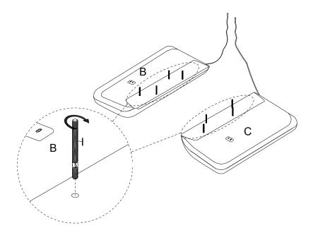
Attach LSF & RSF Arm (B & C) to Back & Seat (A) using Bolt (I), Flat Washer (N), Spring Washer (M) and Nut (L) with Wrench (Q).
