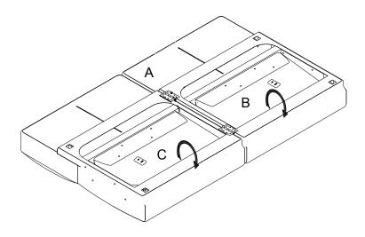
Insert Bolt (I) into LSF & RSF Arm (B & C) by turning clockwise.
