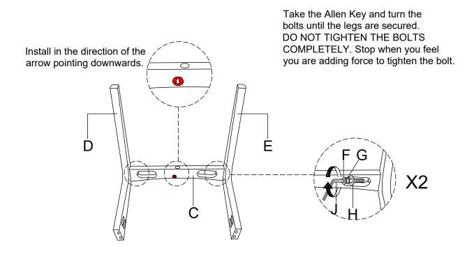
Place the Back Frame (A) on a protective surface. Attach the Back Frame (A) to the Side Leg-LSF & RSF (D & E) using JCBC Bolt (F), Lock Washer (G) and Flat Washer (H) with Allen Key (J).
