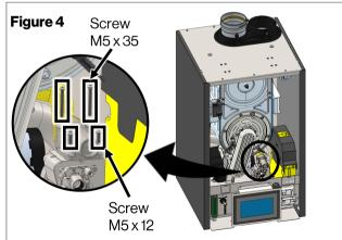
7. Use a 4 mm Allen wrench to remove four screws from the bottom of the unit. Remove the gas valve with two O-rings. Inlet flange stays on the unit and will be reassembled with new gas valve (Figure 5).
