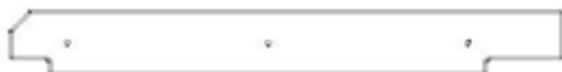
E14 PANNEAU DE REBORD - W4L18720 (x1) 15/16 po x 2 15/16 po x 21 3/4 po (24x74x553)
