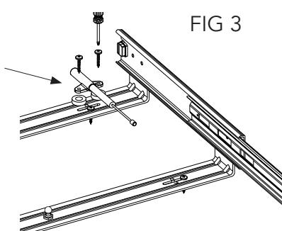
Door thickness must be at least 3/4" where screws attach.
