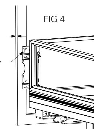
For horizontal adjustment loosen 4 3/8" nuts and move to desired position.
