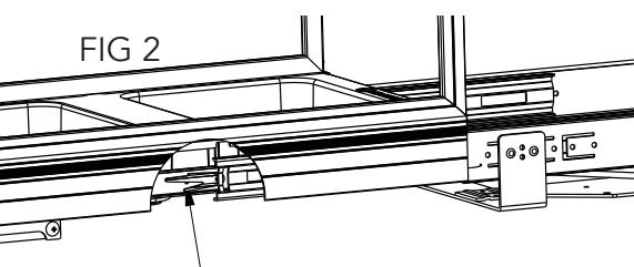
Press release lever behind side skirt on each side by sliding up or down depending on which side. Unit will separate when both levers are disengaged.
