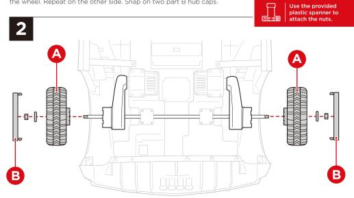
Make sure the rear axle is positioned evenly on the car.
