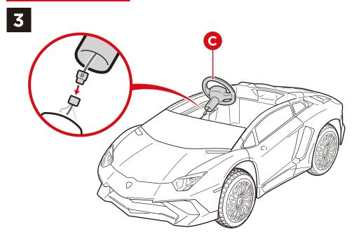
Join the connector from the part C steering wheel to the connector on the steering wheel mount. Slide the steering wheel onto the steering wheel mount.
