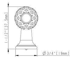
ACCESSORY: SCREW:8-32XI" IPCS BREAK AWAY SCREW:8-32x45 IPCS ALL SCREW MATERIAL:STEEL-SAEI006
