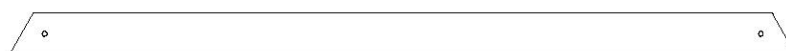
H01 | LISSE DE PLANCHER - W4L16428 (x1) | 1 po x 3 3/8 po x 61 3/4 po (24 x 86 x 1569)
