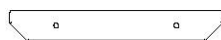
F05 | SUPPORT SUPÉRIEUR - W4L16470 (x2) | 1 3/8 po x 2 3/8 po x 16 3/4 po (36 x 60 x 424)
