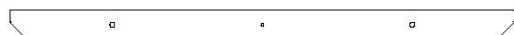
F08 | SUPPORT DE PIED - W4L16472 (x2) | 1 3/8 po x 2 3/8 po x 39 5/8 po (36 x 60 x 1006)
