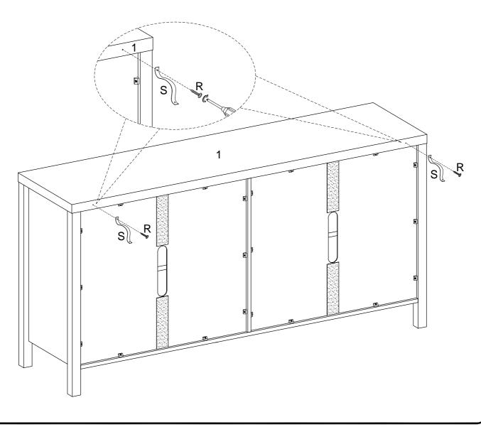
Secure Plastic Strap (S) to wall with Screw (Q) and Wall Anchor (T) as needed depending on your wall type.
