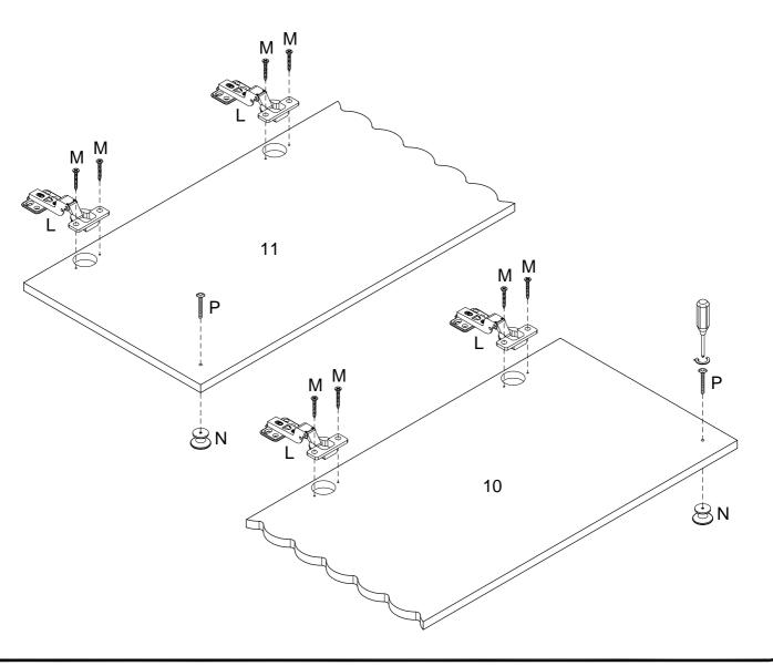
Align attached Hinges (K and L) on Doors (9 and 11) to interior grooves of panels (3 and 5). Secure with Screws (M) with screwdriver.
