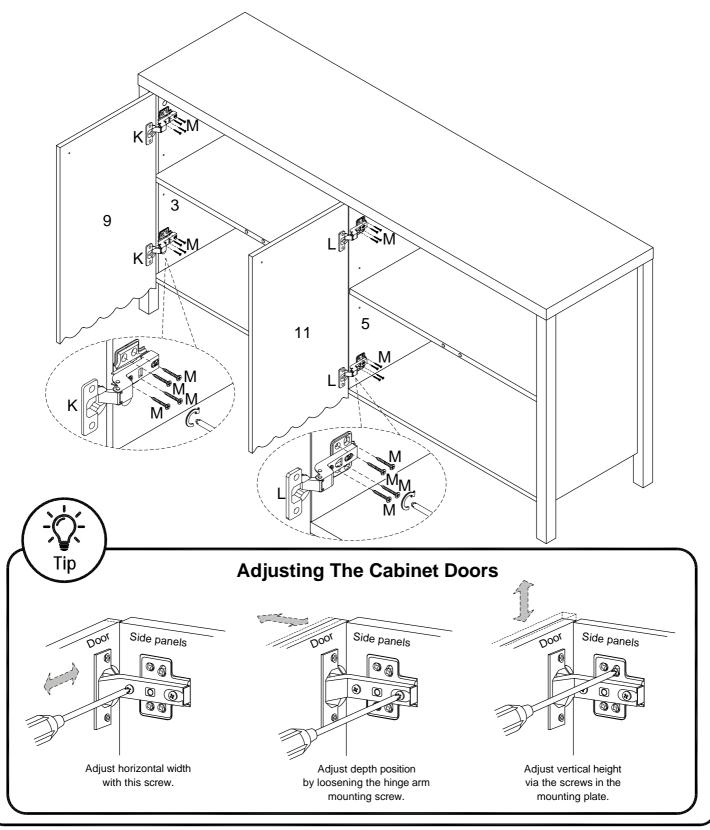
Align attached Hinges (K and L) on Doors (10 and 12) to interior grooves of panels (4 and 5). Secure with Screws (M) with screwdriver.
