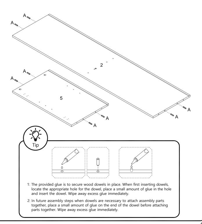
Secure Cam Bolt (B) as indicated below to Top Panel (1), Left Panel (3), and Right Panel (4). Insert Wooden Dowels (A) to ends of Left Panel (3) and Right Panel (4).
