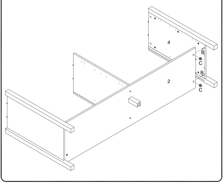
Unfold Back Panels (6). Then align panels with grooves between side panels (3 &4) and middle Divider Panel (5) and slide down to Bottom Panel (2), aligned with grooves.
