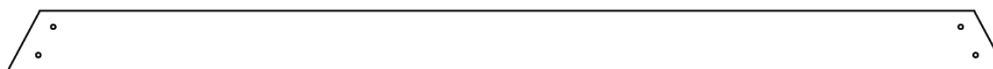
G14 | PLANCHE DE SOL - W4L16019 (x1) 15/16 po x 5 1/4 po x 86 11/16 po (24 x 134 x 2202)
