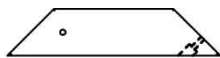
E04 RENFORT D'ANGLE STANDARD - W4L16342 (x4) 1 3/8 po x 2 3/8 po x 13 po (36 x 60 x 330)
