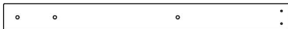
M28 | PANNEAU MURAL - W4L16064 (x1) 5/8 po x 3 3/8 po x 35 po (16 x 86 x 888)
