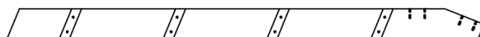
E75 | MONTANT DROIT - W4L16029 (x1) | 1 3/8 po x 3 3/8 po x 50 3/4 po (36 x 86 x 1290)
