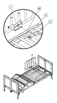
For easier installation, the end of the threaded ຶ່ງ rod on the "T" bracket  ${\ensuremath{\mathbb K}}$  should be inside the outer edge  $\mathbb{N}$  of the bed frame.
