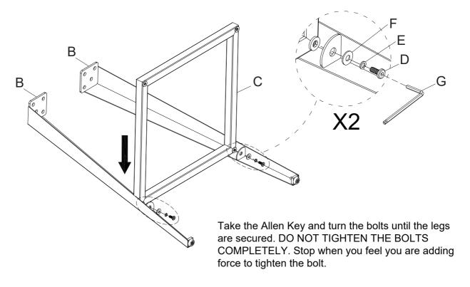
Attach the other 2pcs Metal Leg (B) to the Footrest Frame (C) using Bolt (D), Spring Washer (E) and Flat Washer (F) with Allen Key (G).
