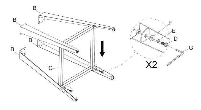
Attach the Metal Leg (B) to the Wood Seat (A) using Bolt (D), Spring Washer (E) and Flat Washer (F) with Allen Key (G).
