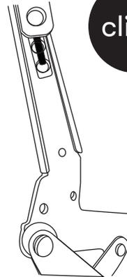
Firmly push each side into place one at a time. **You should hear a click** when the chair back locks into place on each side.
