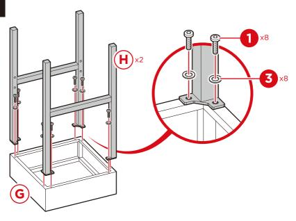
Attach two part I supports with eight part 1 screws and eight part 3 washers.
