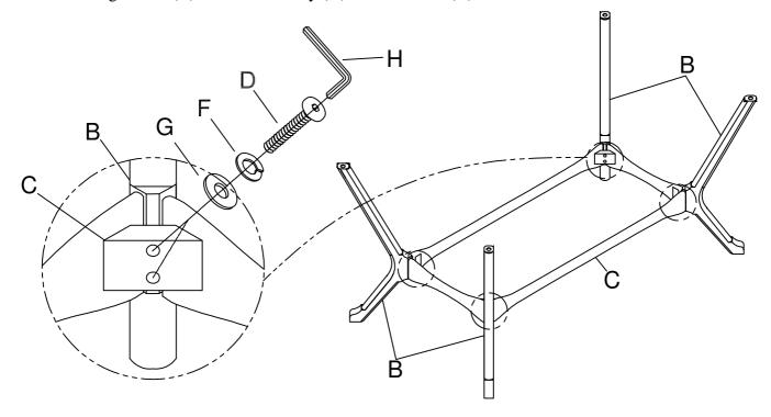
Attach Leg Frame (C) to Table Top (A). Use Allen Bolt (E), Lock Washer (F) and Flat Washer (G) on holes of Table Top (A). Turn Allen Key (H) in Allen Bolt (E).
