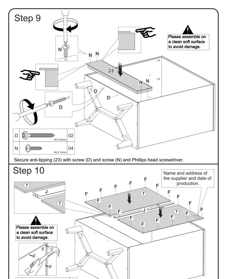
Secure back panel (7) with part (J) to body with nails (F).
