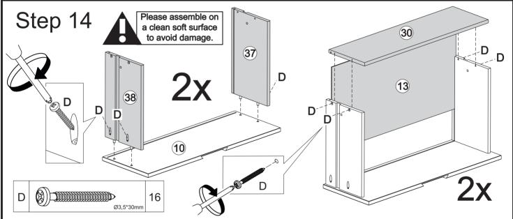
Secure part (37) and (38) to part (10) with screw (D) and Phillips head screwdriver. Insert part (13) between parts (37) and (38). Attach part (30) to parts (37) and (38) with screws(D) and Phillips head screwdriver.
