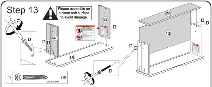
Secure part (32) and (41) to part (15) with screw (D) and Phillips head screwdriver. Insert part (13) between parts (32) and (41). Attach part (29) to parts (32) and (41) with screws(D) and Phillips head screwdriver.
