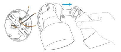
Floodlight Wired must be installed on a 4" round UL listed junction box. If you don't have an existing junction box, you'll need to hire a licensed electrician to install one. Be sure to comply with your local building codes.
