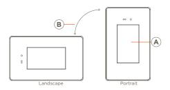
LCD Touchscreen - The display is a multicolored touchscreen LCD that includes various screens for viewing and configuring the HVAC system.
