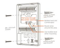
IMPORTANT! As indicated in the diagram above, route the thermostat wires around the wiring keepout. When the two halves of the thermostat are snapped together the component that rests in that indented area could be damaged.
