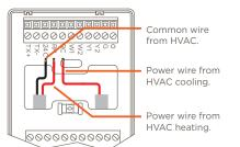
$\mbox{\bf RH}$  - Supplies power to the relays connected to terminals W1, W2, and O.
