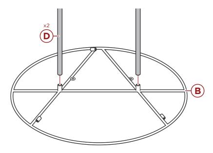
Locate the part J legs/feet and insert the part D inner poles, then secure the feet to the part B base stand with two part 2 zip ties.
