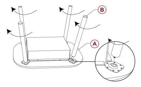
Peel the paper off the back of one part G table leg bottom protector and attach it to one part B table leg. Repeat to attach three more bottom protectors.
