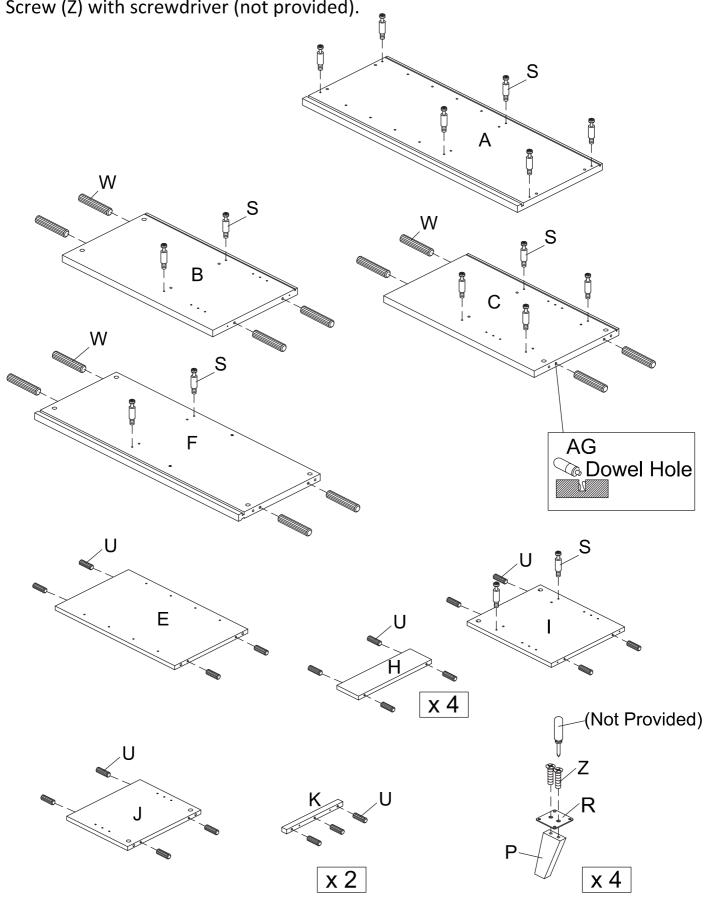
Insert Cam (T) into Top Shelf Panel (E). Attach Big Top Divider Panel (I) to Top Shelf Panel (E) using Cam (T) with screwdriver (not provided). Apply Glue (AG) to the Dowel Holes of Top Shelf Panel (E). Then attach Small Top Divider Panel (H) to Top Shelf
