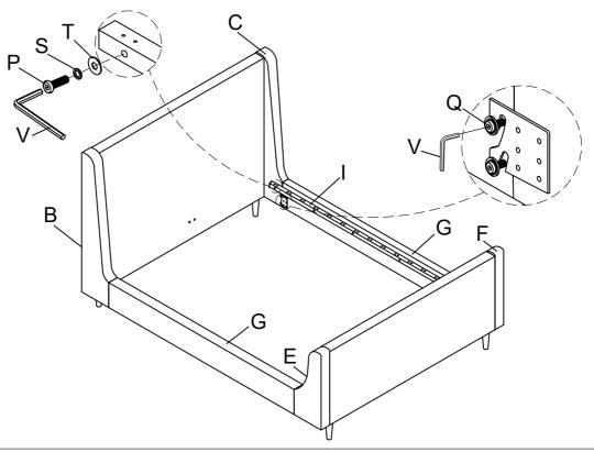
Attach Middle Rail (H) to Headboard Panel (A) & Footboard Panel (D), using Bolt (Q), Lock Washer (S) and Flat Washer (T) by Allen Key (V) as below shown.
