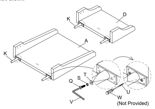
4 Attach Bolt (Q), Lock Washer (S) and Flat Washer (T) to Hardboard Side - LSF (B), Hardboard Side - RSF (C), Footboard Side - LSF (E) & Footboard Side - RSF (F) by Allen Key (V) as below shown. But not too tight.
