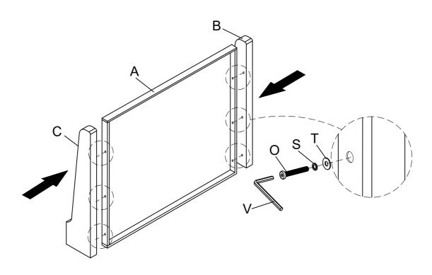
2 Attach Footboard Panel (D) to Footboard Side - Left (E) & Footboard Side - RSF (F), using Bolt (O), Lock Washer (S) and Flat Washer (T) by Allen Key (V).
