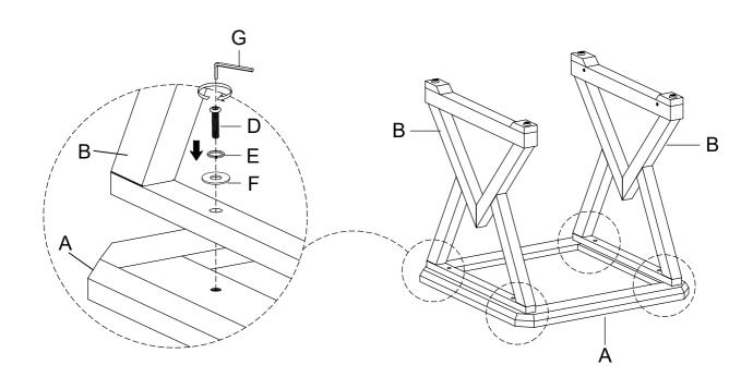
2 Attach the Shelf (C) to the Leg Frame (B) using Bolt (D), Spring Washer (E) and Flat Washer (F) with Allen Wrench (G). Fully tighten the bolts in this step.
