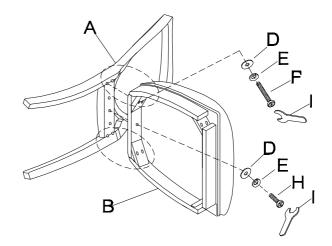
Attach Chair Leg(C) to Seat Cushion(B), insert Bolt(G), SpringWasher(E), Flat Washer(D) and tighten with Allen Wrench(I).
