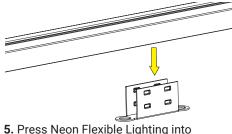
Press Neon Flexible Lighting into Bottom Mounting Clips for a secure installation.
