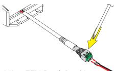
Use a T-FBC Female Barrel Connector to connect the starter wire to receiver or power supply; match Red to Red and Black to Black to maintain polarity.
