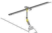
Use a drill or screwdriver to install Loop Mounting Clips in desired locations.
