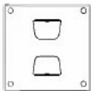
G1 | POST FOOT PLATE - A4M01278 (4) | 2 1/8"x8 3/8"x8 3/8" (54x213x213)
