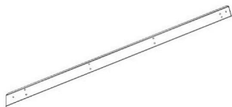
E01 PLANCHE DE NOUE - W4L21712 (x2) 1 7/16 po x 3 3/8 po x 82 15/16 po (36 x 86 x 2104)
