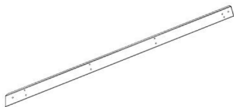
E01 PLANCHE DE NOUE - W4L21712 (x2) 1 7/16 po x 3 3/8 po x 82 15/16 po (36 x 86 x 2104)
