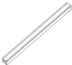
P01 POTEAU - W2A04716 (x2) 6 po x 6 po x 89 1/2 po (152 x 152 x 2274)
