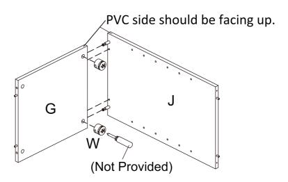
Insert Cam (W) into Left Bottom Divider Panel (J). Apply Glue (AK) to the Dowel Holes of Shelf (H). Then attach Shelf (H) to Left Bottom Divider Panel (J) using Cam (W) with screwdriver (not provided) and cover Cam (W) by Sticker (AJ).
