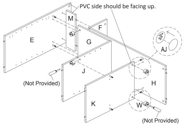
Insert Cam (W) into Shelf (H) and Right Shelf Panel (I). Then attach Shelf (H) and Right Shelf Panel (I) to Right Side Panel (C) and Right Bottom Divider Panel (K) using Cam (W) with screwdriver (not provided). Apply Glue (AK) to the Dowel Holes of Left Side Panel (B) and Middle Side Panel (E). Then attach Wine Rack Shelf Panel (M) to Left Side Panel (B) and Middle Side Panel (E).
