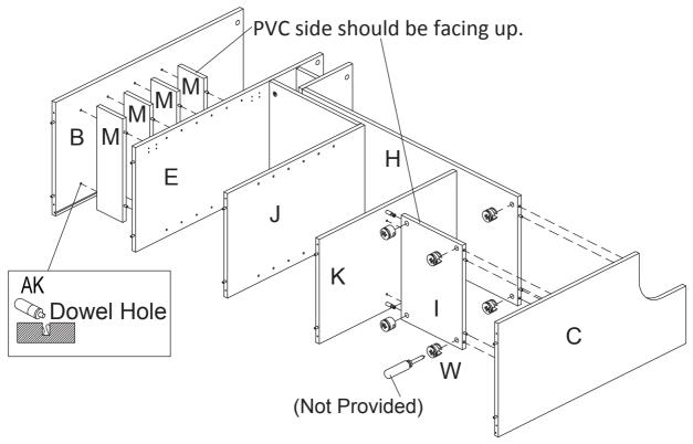
Insert Cam (W) into Left & Right Side Panel (B & C), Middle Side Panel (E) and Top Divider Panel (F). Then attach Top Panel (A) to Left & Right Side Panel (B & C), Middle Side Panel (E) and Top Divider Panel (F) using Cam (W) with Allen Wrench (AI) and screwdriver (not provided) and cover Cam (W) by Sticker (AJ).
