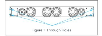
2. Secure to the surface using the appropriate screws for the surface material, ensuring proper positioning and leveling.
