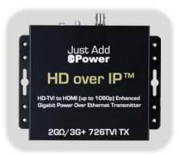
**Mix-and-match!** The  $2G\Omega/3G$  + TVI POE Transmitter is fully compatible with all  $2G\Omega/3G$  and 3G devices. Add an HD-TVI source to your HD over IP system without the need for a TVI-HDMI converter.
