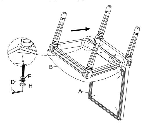
3 Finally, assemble the last Bolt (F) to Seat (B) and Chair Back (A) with Lock Washer (D) & Flat Washer (E) by Allen Key (I).
