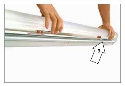
3. Rotate lens counterclockwise to release from rear reflector.
