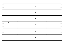
HH5 FLOOR PANEL - W2A03076 (x1) | 1 1/4"x20 9/16"x32 7/16" (32x522x824)
