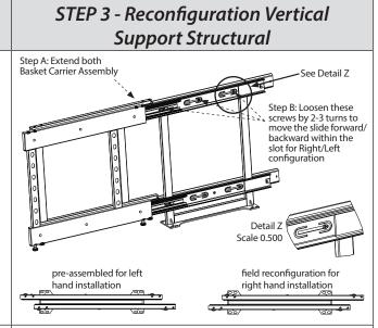
First extend the Basket Carrier Assembly to gain access and loosen the screws in View Z by 2-3 turns, and slide to Right Hand configuration.
