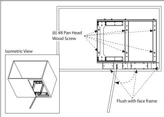
Position the Roller Guide Bracket and Installation Hinge Spacer against the back of the face frame or 3/4" behind opening on frameless application. Install completed Base Assembly to the cabinet floor with (6) #8 Pan Head Wood screw. Remove all tie wraps securing the assembly.
