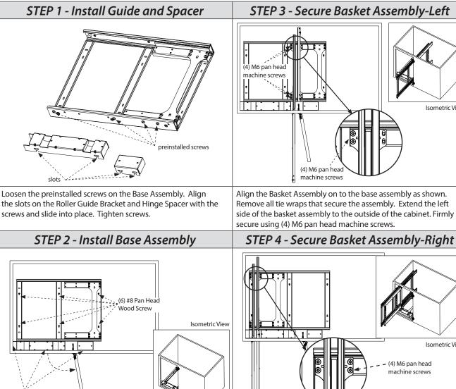
Position the Roller Guide Bracket and Installation Hinge Spacer against the back of the face frame or 3/4" behind opening on frameless application. Install completed Base Assembly to the cabinet floor with (6) #8 Pan Head Wood screw. Remove all tie wraps securing the assembly.
