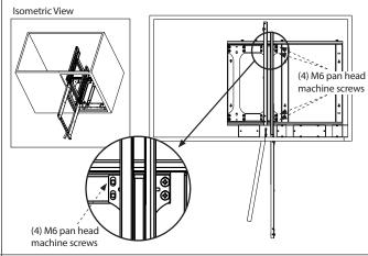
With the right Basket Carrier Assemblies extended outside of the cabinet, tighten with the M6 pan head machine screws. Then, slide the Vertical Support Assembly to the right side and extend the left Basket Carrier out of the cabinet. Tighten with M6 pan head machine screws.
