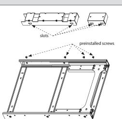
Loosen the preinstalled screws on the Base Assembly. Align the slots on the Roller Guide Bracket and Hinge Spacer with the screws and slide into place. Tighten screws.
