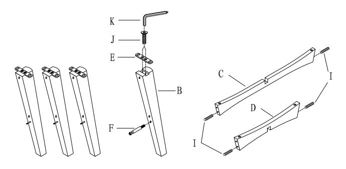
Insert Wood Dowel (I) into the pre-drilled holes of the cross bar of Top Panel (A) as shown below, then attach one Leg (B) to Top Panel (A) by using Bolt (J) with Allen Key (K).
