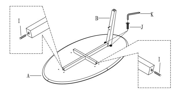
Attach Long Cross Bar (C) to assembled Leg (B) by using Cam Nut (H) and Cam Screw (G) with Allen Key (K) as shown below, then attach another Leg (B) to Long Cross Bar (C) by using Cam Nut (H) and Cam Screw (G) with Allen Key (K), then lock Leg (B) into Table Top (A) by using Bolt (J) with Allen Key (K) as drawing below.
