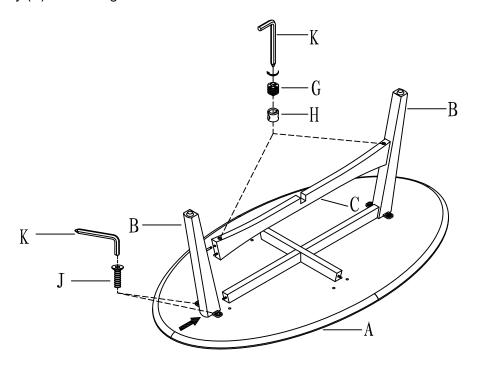
Attach Short Cross Bar (D) to Long Cross Bar (C), then assemble another two Legs (B) into Short Cross Bar (D) by using Cam Nut (H) and Cam Screw (G) with Allen Key (K) as shown below, then lock Leg (B) into Table Top (A) by using Bolt (J) with Allen Key (K) as drawing below.
