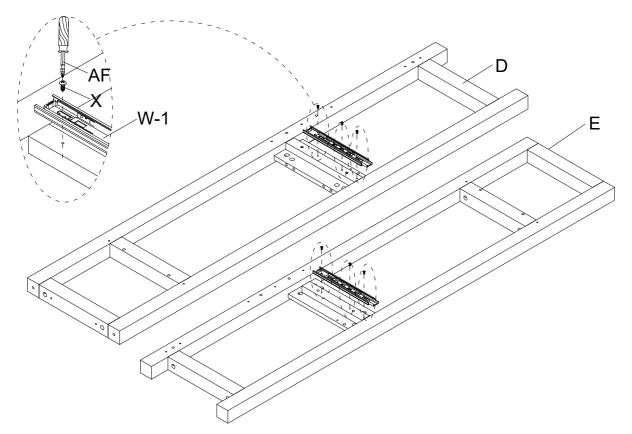
4 Insert Bolt (S) into Left Side Frame (D) and Right Side Frame (E) by Screwdriver (AF) as below shown.
