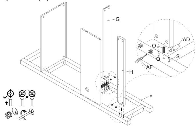
7 Assemble Left Side Frame (D) to pre-assembled Bottom Support Panel (G) and Back Bottom Panel (H), Back Panel (F) and Shelf Panel (B), using Glue (AD) & Wood Dowel (O) first, then attach Nut (Q) to Bolt (S) by Screwdriver (AF) as below shown.
