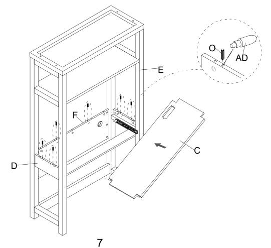
**11** Put Desk Box Top (C) to the top of Back Panel (F), Left side frame (D) and Right Side Frame (E) using Nut (Q) by Screwdriver (AF) as below shown.
