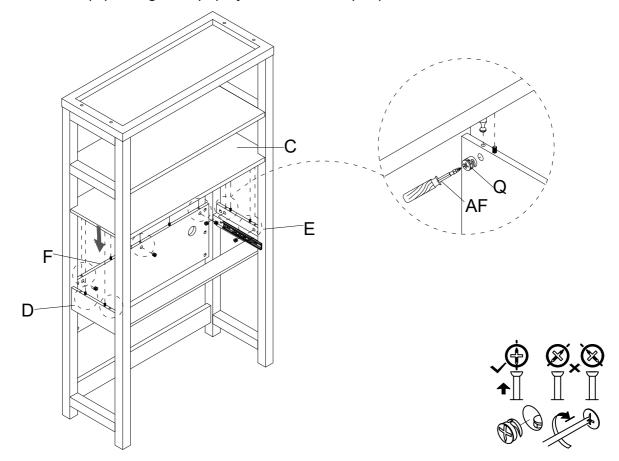
12 Attach Adaptor (U) to the hole of Desk Box Top (C), using Screw (V) by Screwdriver (AF) as below shown.
