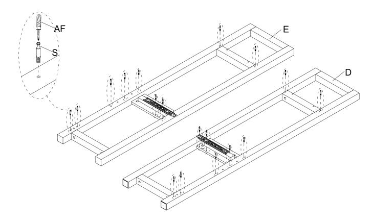
5 Assemble Back Panel (F) and Shelf Panel (B) to Right Side Frame(E), using Glue (AD) & Wood Dowel (O) first, then attach Nut (Q) to Bolt (S) by Screwdriver (AF), put Grommet (AE) to Back Panel (F) as below shown.
