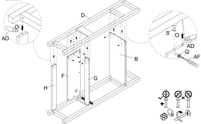
8 Assemble Back Bottom Panel (H) to Side Frame (D), using Nut (Q) by Screwdriver (AF) as below shown.
