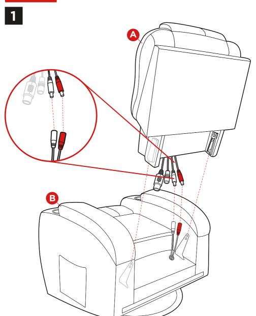
Insert part A backrest into part B seat, ensuring the two metal inserts on the seat slide into the clips on the backrest with a click. Join the wires from the backrest to the corresponding wires on the seat. Make sure that the corresponding sizes and colors match.
