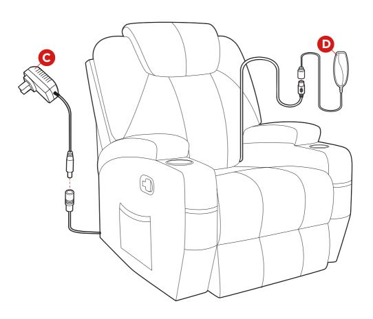
Join the part C wall adaptor plug and part D remote to the appropriate wires.
