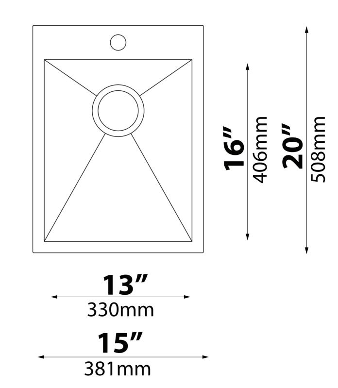
**NOTE:** Cutout template is provided as a guide **ONLY** and must be checked against actual sink to verify correct fit.
