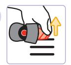
Pull Buckle and Buckle Cover Out of Shell
