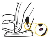
There is a small window on both sides of the car seat that displays the current position.
