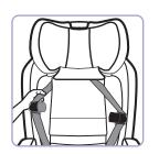
Slide Shoulder Harness Straps Out from Slots in Headrest Pad
