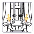
Lift Bottom of Headrest Pad Up and Undo Both Fasteners on Lower Back of Seat Pad
