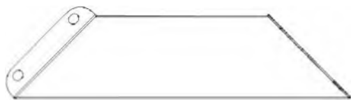
C01 ASSEMBLAGE DE CORBEAU - A4M03525 (x1) 21 13/16" x 5 1/4" x 2 3/4" (70x134x553.5)
