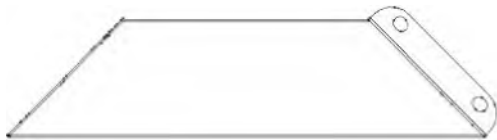
C02 ASSEMBLAGE DE CORBEAU - A4M03526 (x1) 21 13/16"x5 1/4"x2 3/4" (70x134x553.5)
