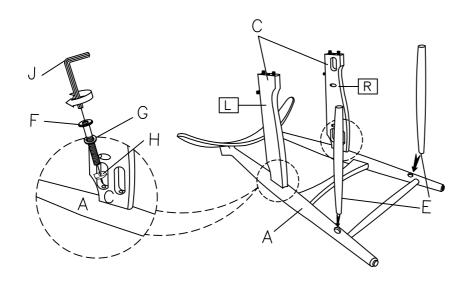
Take the Allen Wrench, and turn the bolts until the legs are secure. DO NOT TIGHTEN COMPLETELY.
