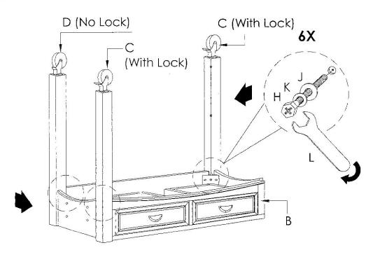
Align the hole of corner block of Shelf (E) to the holes of Leg (C & D). Tighten the Shelf (E) with Flat Washer (J), Spring Washer (K) and Hex Bolt (H) using Wrench (L).
