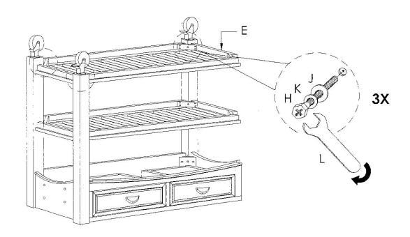
Place the last Leg (D) to the corner of Apron and tighten it with Flat Washer (J), Spring Washer (K) and Hex Bolt (H) using Wrench (L).
