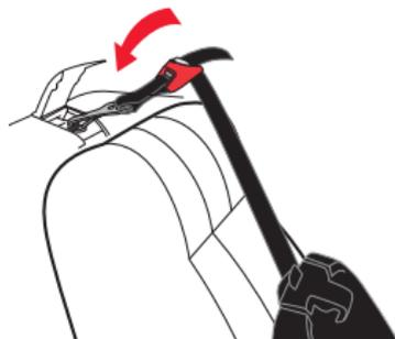
4. Attach LATCH/UAS Connectors to vehicle Lower Anchor Bars. Connectors will make an audible **CLICK** when attached on both sides of the base. Make sure they are attached by pulling firmly on connectors.
